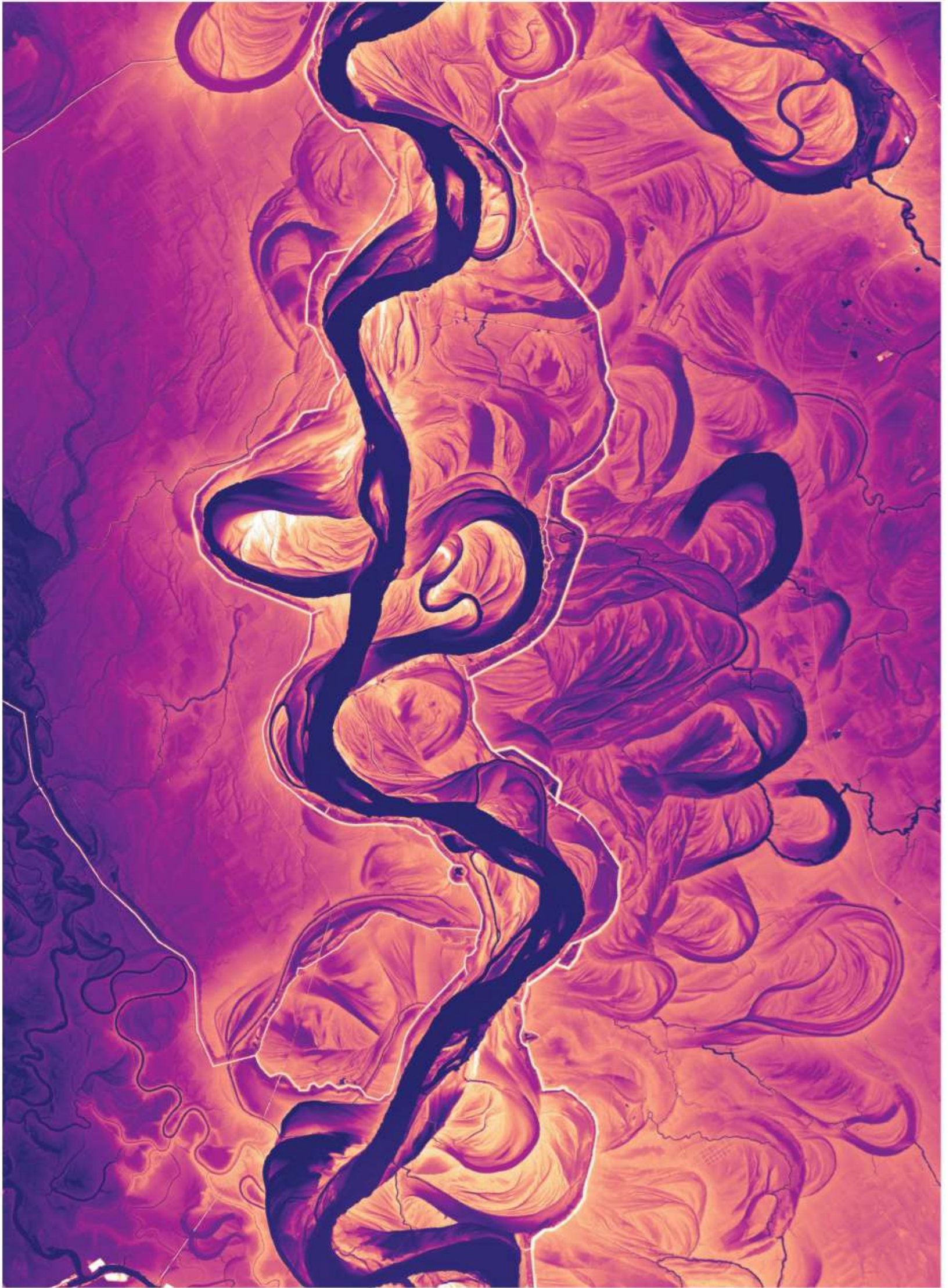
By comparison, a map created using lidar shows shifts over the past 75 years. Erosion and changes in flow caused the channel to widen in the middle of the image and migrate toward the south.
